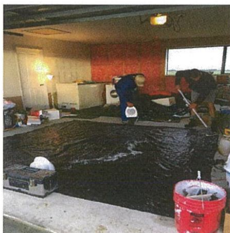
Left 4: Covers from plots being swept to recover the fine particles for weighing to confirm the calibration of the truck application.
