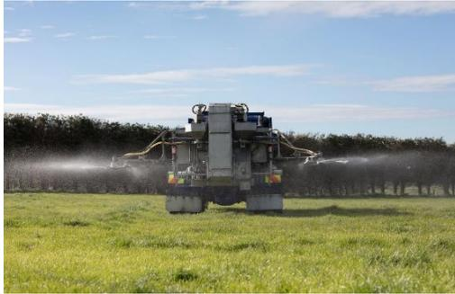
P 2: FPA truck applying fertiliser in fine particle form
