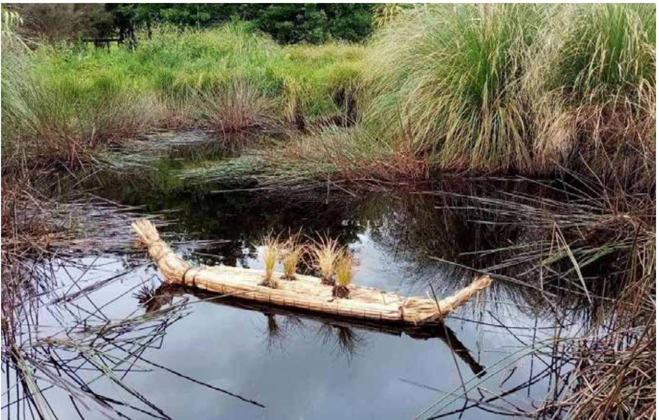
Living Water supported Ngāti Apakura with their innovative trial of a mōkihi - a natural floating wetland, constructed from raupō and harakeke flower stalks - to treat nutrients at Lake Ruatuna.
