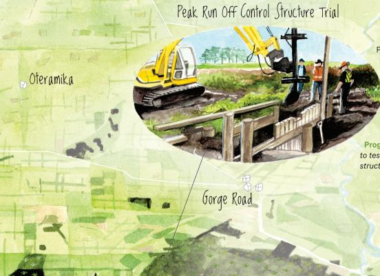
Peak run-off control structures are being trialled in the Carran Creek catchment where small dam-like structures are built in drains to temporarily pond water, providing more time for contaminants to drop out before being carried downstream, and lessen the intensity of flows to reduce bank erosion.
