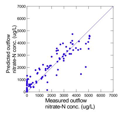
**Figure 7-7:** Comparison of woodchip filter measured and predicted nitrate-N outflow concentrations. The predicted concentrations were derived from measured inflow concentrations using Equation 2-3 described in section 2.5.2. The statistical relationship between measured and modelled values is described in Appendix J.
