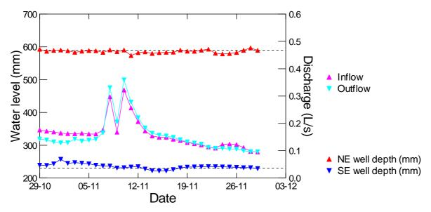
**Figure 7-22:** Time-series of daily average inflows and outflows, and water levels in the woodchip filter, recorded in the NE (inlet) SE (outlet) corner of the bed. Results for two closely spaced minor inflow events during November 2017 are shown. These are daily average flows derived from five-minute data. The broken horizontal lines are for visual reference purposes.
