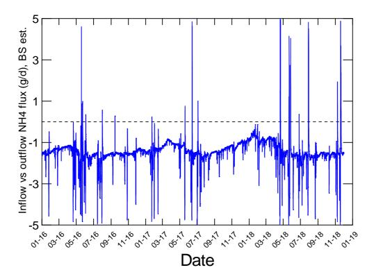
**Figure J-10:** Performance of the woodchip filter in terms of ammoniacal-N removal, grams per day. Negative values indicate that the filter is a net source of ammoniacal-N. The spikes are artefacts of timing differences between the two models.
