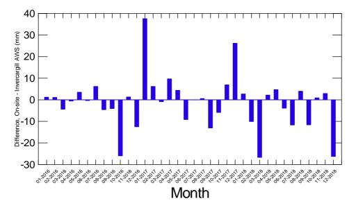
**Figure D-3:** Difference between monthly total rainfall measured on site with rainfall measured at **Invercargill airport.** Data sourced from "Invercargill Aero AWS", Site 684305.
