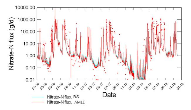
**Figure 7-6:** Nitrate-N outflow flux from woodchip filter, estimated using two models. The red dots indicate instantaneous flux estimated from grab samples used to calibrate the models. BS=bootstrap regression model, AMLE = model from LOADEST modelling package (Runkel et al. 2013).
