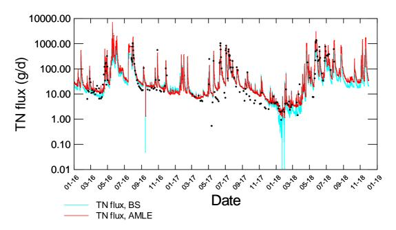
**Figure J-15: TN outflow flux from the woodchip filter, estimated using two models.** The black dots indicate instantaneous flux estimated from grab samples used to calibrate the models. BS=bootstrap regression model, AMLE = model from LOADEST modelling package (Runkel et al. 2013).
