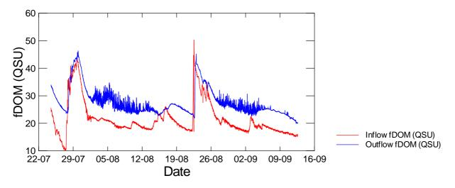
**Figure 5-5:** Comparison of inflow and outflow fluorescent dissolved organic matter concentrations. Fluorescent dissolved organic matter concentrations are reported in quinone sulphate units (QSU).
