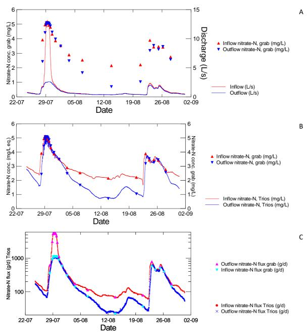
**Figure 5-1:** Inflow and outflow nitrate-N concentrations and flux. A) Grab sample concentrations for July and August 2018, B) five-minute TriOS nitrate-N estimates of nitrate-N and grab sample concentrations, and C) instantaneous nitrate-N load derived from TriOS measurements and grab sample concentrations. Note the y-axis in C) has a log<sub>10</sub> scale.
