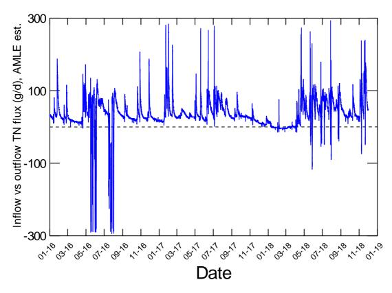
Figure J-17: TN removal by woodchip filter - inflow minus outflow TN flux, estimated using bootstrap regression models.
