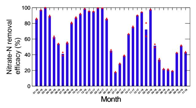
**Figure 7-16:** Average nitrate-N removal efficacy, estimated as the percent of inflow flux removed by the filter by month. The inflow flux was estimated using the LOADEST AMLE model, and the outflow flux was estimated from inflow concentrations using the process model described in section 2.5.2. These data were derived from hourly estimates. The red triangles indicate the 95% lower and upper confidence intervals of the monthly mean values.
