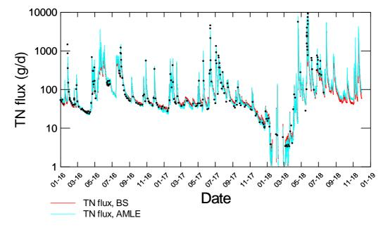
**Figure 7-20: TN inflow flux to the woodchip filter, estimated using two models.** The black dots indicate instantaneous flux estimated from grab samples used to calibrate the models. BS=bootstrap regression model, AMLE = model from LOADEST modelling package (Runkel et al. 2013).
