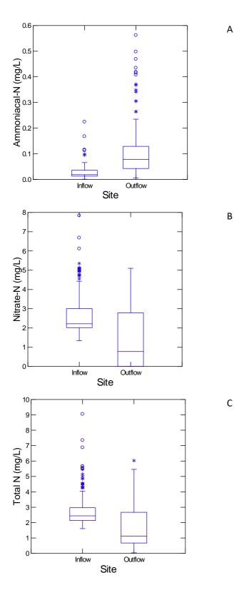
**Figure J-2:** Comparison of inflow and outflow concentrations for all grab samples (mg/L). A= Ammoniacal- N, B= Nitrate-N C= Total N.
