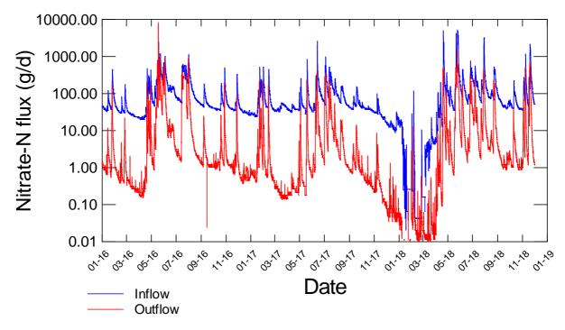
Figure J-13: Time-series of hourly average inflow and outflow nitrate-N flux derived from two bootstrap regression models. These are hourly average values derived from five-minute data.
