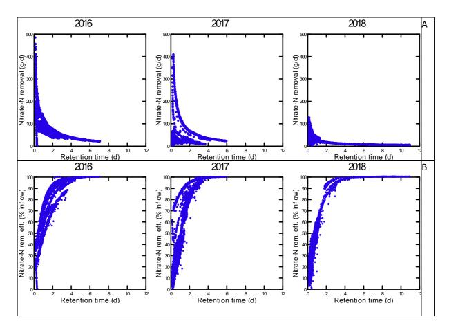
**Figure K-6:** Relationship between nitrate-N removal performance and retention time by year. A) Nitrate-N removal rate (g/d), and B) nitrate-N removal efficacy in terms of proportion of influent load removed.
