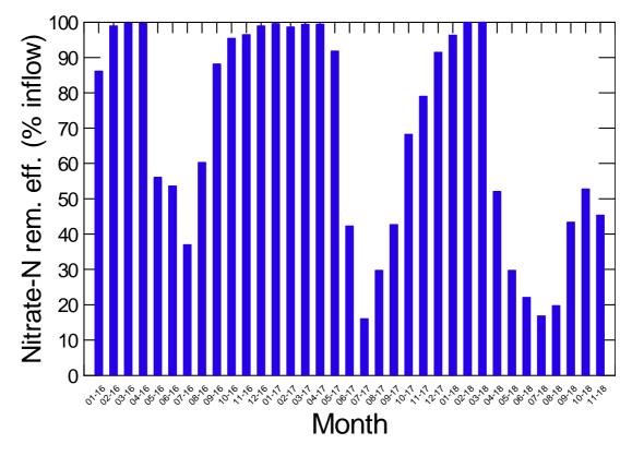
Figure K-2: Median nitrate-N removal efficacy, estimated as the percent of inflow flux removed by the filter by month.
