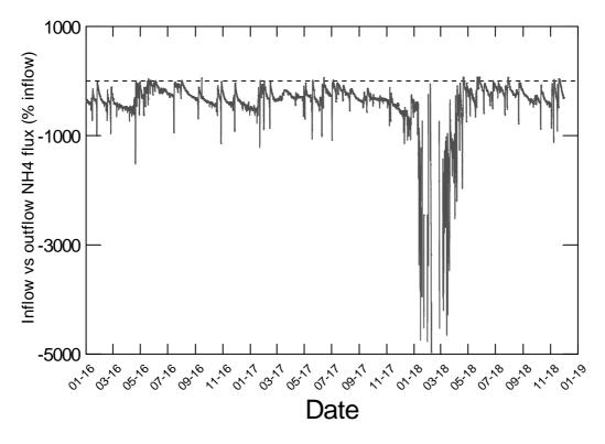
**Figure J-11: Performance of the woodchip filter in terms of ammoniacal-N removal, reported as proportion of inflow load.** Negative values indicate that the filter is a net source of ammoniacal-N. The spikes and large negative values are artefacts of timing differences between the two models and extremely low flows that occurred in summer 2017/2018.
