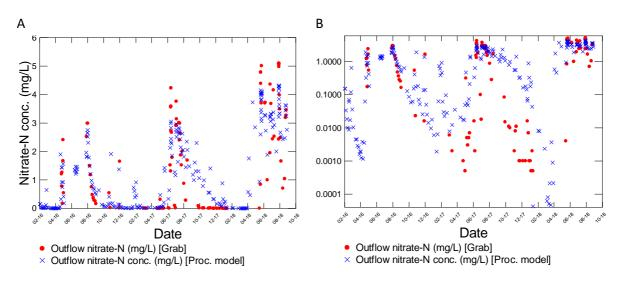
**Figure 7-8:** Time series of measured (red dots) and predicted (blue crosses) woodchip filter nitrate-N outflow concentrations at normal (A) and log<sub>10</sub> scale (B). The predicted concentrations were derived from the measured inflow concentrations using the process-based model (Equation 2-3) described in section 2.5.2. The statistical analysis of measured and modelled values is described more fully in Appendix J.
