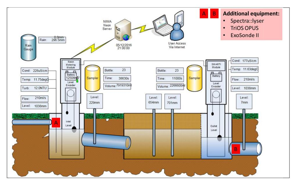
Figure A-1: Schematic from NEON logger schema indicating location and type of measurement equipment. A and B indicate location and type of additional equipment.
