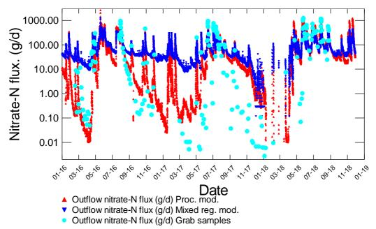
**Figure 7-9:** Time series of measured and predicted woodchip filter nitrate-N outflow flux. Note the y-axis has log<sub>10</sub> scale. The measured flux was derived from grab sample results. The predicted flux was derived from the measured inflow concentrations using the process model equation described in section 2.5.2 (Proc. Mod.), and from the mixed regression model previously described (Mixed reg. mod.).
