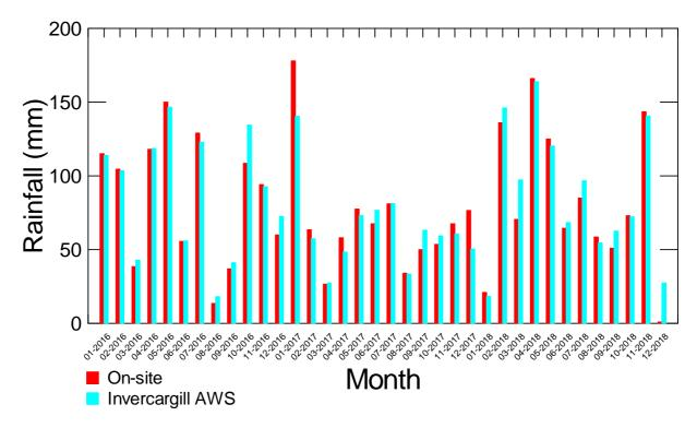
**Figure D-2:** Comparison of on-site monthly total rainfall, 2016-2018 inclusive, with rainfall recorded at **Invercargill airport.** Data sourced from "Invercargill Aero AWS", Site 684305.
