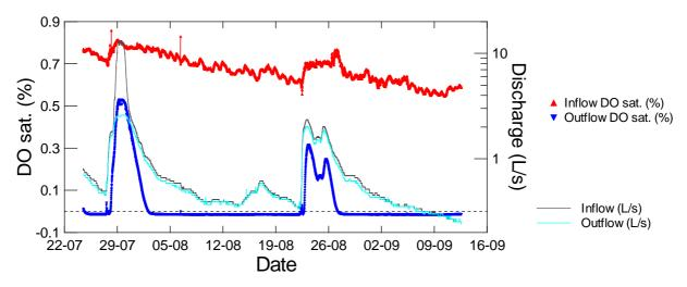
**Figure 5-4:** Comparison of inflow and outflow dissolved oxygen concentrations, and relationship to inflow events. Dissolved oxygen concentrations are expressed in terms of percent saturation.
