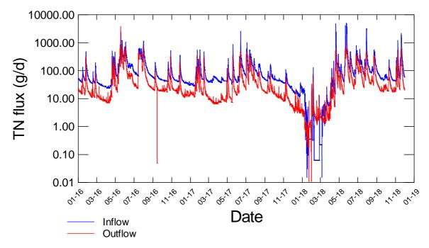
Figure 7-21: Comparison of woodchip filter inflow and outflow TN flux estimated using bootstrap regression models.
