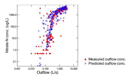
**Figure J-7:** Relationship of measured and process-model predicted outflow nitrate-N concentrations and flow, all values. Note that concentrations and flows are expressed as log<sub>10</sub> values.
