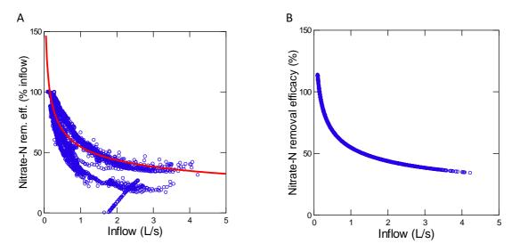
**Figure 7-18:** Relationship between nitrate-N removal performance and inflow, 2016 data only. Left) model fitted to data, and Right) model that could be used to guide design.
