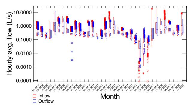
**Figure E-1:** Hourly average flow recorded for woodchip inflow and outflow. Data derived from five-minute data.
