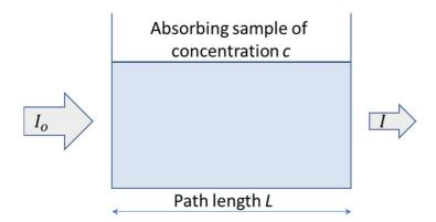
where  $I_o$  is the **initial light intensity** and I is the **light intensity** after it passes through the sample.
