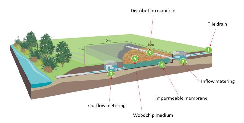
Figure 2-3: Schematic of nitrate-N filter showing dimensions and key components of the as-built filter.
