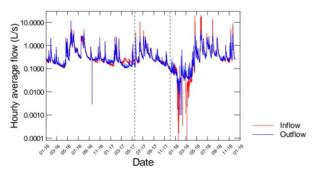
**Figure 4-1:** Comparison of inflow to and outflow from the woodchip filter. Hourly average flows were derived from five-minute data. Note *y*-axis has log<sub>10</sub> scale.
