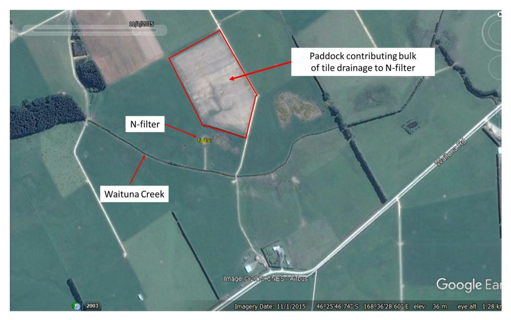
**Figure 2-2:** Location of nitrate-N filter relative to the paddock which is the principal source of shallow groundwater draining into the filter. Waituna Creek flows from right to left.
