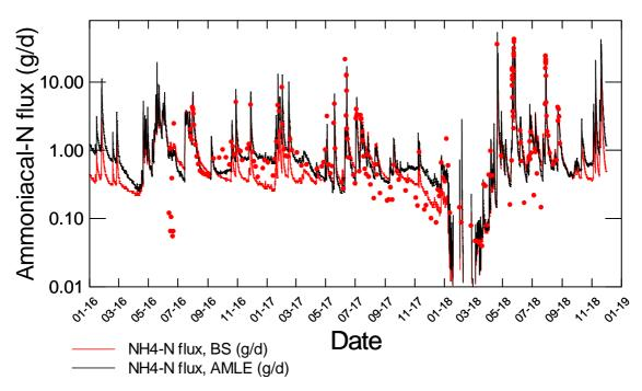
**Figure 7-1: Ammoniacal-N inflow flux to woodchip filter, estimated using two models.** The red dots indicate instantaneous flux estimated from grab samples used to calibrate the models. BS=bootstrap regression model (Rutherford, pers. comm.), AMLE = model from LOADEST modelling package (Runkel et al. 2013).
