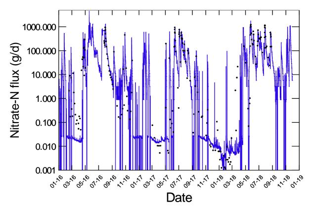
**Figure J-12:** Time-series of hourly average outflow nitrate-N flux derived from a mixed regression model. The black dots are grab sample flux estimates. The spikes <0.001 are artefacts of the calculation process, and were removed from the performance calculations. These are hourly average values derived from five-minute data.
