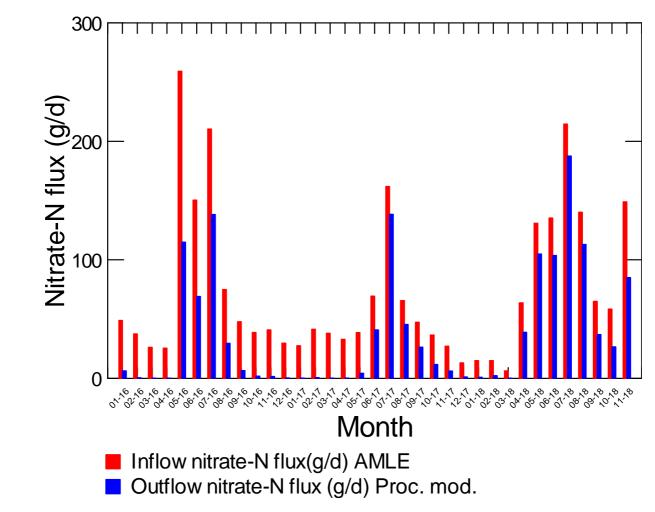
**Figure 7-14:** Comparison of median nitrate-N inflow and outflow flux by month. The inflow flux was estimated using the LOADEST AMLE model, and the outflow flux was estimated from inflow concentrations using the process described in section 2.5.2.
