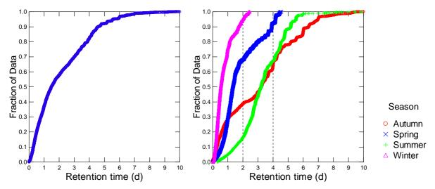
**Figure 4-3:** Distribution of theoretical retention time in the woodchip filter (left), and relationship between retention time and season (right). Note that x-axis of figure on right has log<sub>10</sub> scale. The dashed vertical lines indicate two- and four-day retention time respectively.
