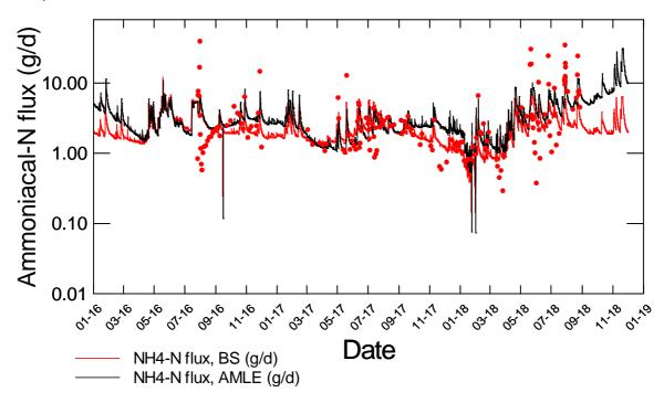
**Figure 7-2:** Ammoniacal-N outflow flux from woodchip filter, estimated using two models. The red dots indicate instantaneous flux estimated from grab samples used to calibrate the models. BS=bootstrap regression model, AMLE = model from LOADEST modelling package (Runkel et al. 2013).
