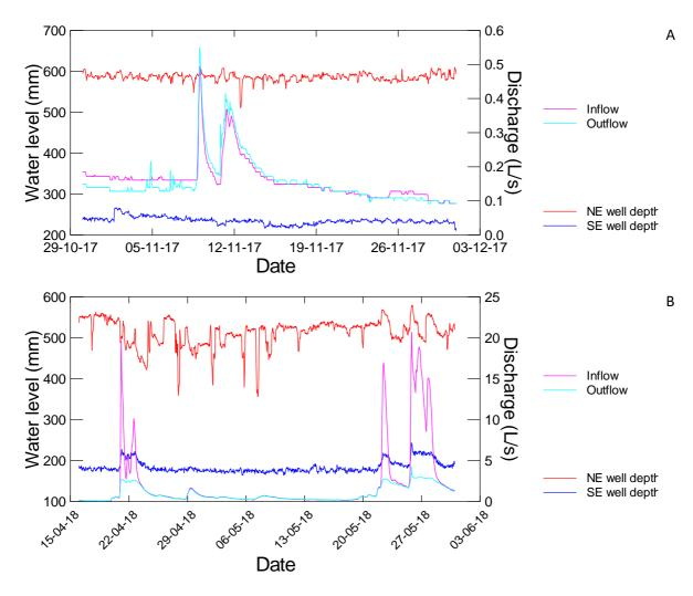
**Figure G-1:** Time-series of hourly average inflows and outflows, and water levels in the woodchip filter, recorded in the NE (inlet) SE (outlet) corner of the bed. A) shows results for two closely spaced minor inflow events (November 2017), and B) shows the results for a series of much larger events in autumn 2018. These are hourly average values derived from five-minute data.
