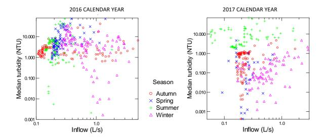
**Figure I-1:** Relationship between daily median turbidity and woodchip inflow classified according to season. These values were derived from five-minute data. Note x axis scales are different. Both x– and y- axes have log<sub>10</sub> scale.
