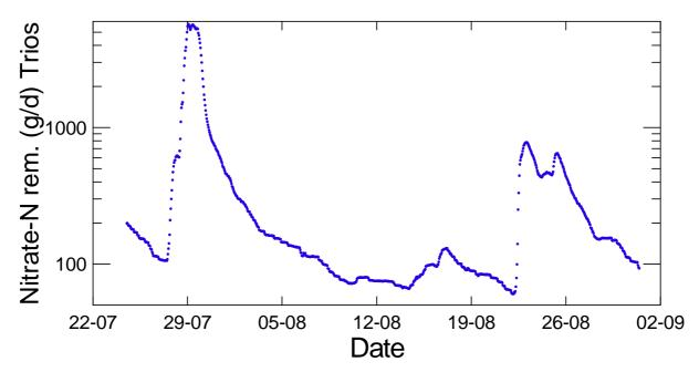
**Figure 5-2:** Estimate of nitrate-N removal efficacy derived from TriOS inflow and outflow measurements. The removal efficacy is the difference between the inflow and outflow mass load estimated at five-minute intervals.
