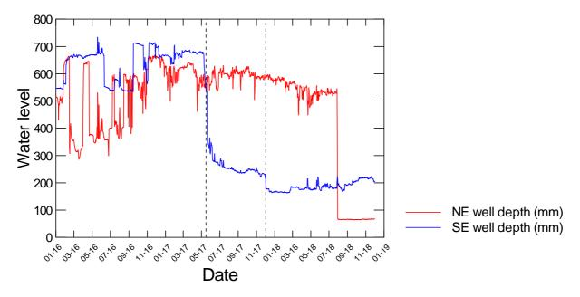
**Figure 4-2:** Time-series of water levels in the woodchip filter, recorded in the NE (inlet) SE (outlet) corner of the bed. These are daily average values derived from five-minute data. The vertical broken lines indicate 15/05/2017 and 1/12/2017 respectively. The inlet recorder was disabled in August 2018.
