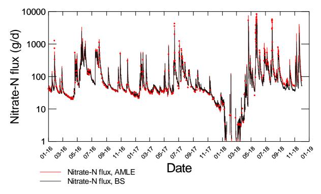
**Figure 7-5:** Nitrate-N inflow flux to woodchip filter, estimated using two models. The red dots indicate instantaneous flux estimated from grab samples used to calibrate the models. BS=bootstrap regression model, AMLE = model from LOADEST modelling package (Runkel et al. 2013).
