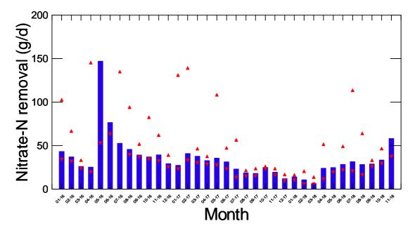
**Figure 7-15:** Median nitrate-N removal, estimated as the difference between inflow and outflow flux by month. The inflow flux was estimated using the LOADEST AMLE model, and the outflow flux was estimated from inflow concentrations using the process model described in section 2.5.2. These data were derived from hourly estimates. The red triangles indicate the 10<sup>th</sup> and 90<sup>th</sup> percentile values.
