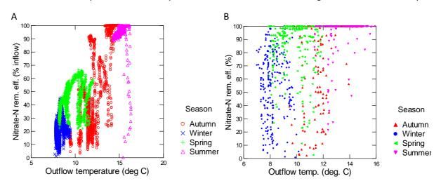
**Figure 7-19:** Influence of temperature on nitrate-N removal performance. A) Performance data derived from the process model, B) performance data derived from the regression model.
