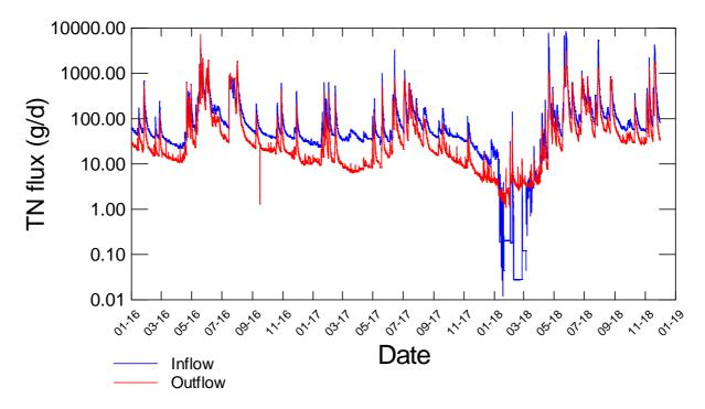
Figure J-16: Comparison of woodchip filter inflow and outflow TN flux estimated using AMLE regression models.
