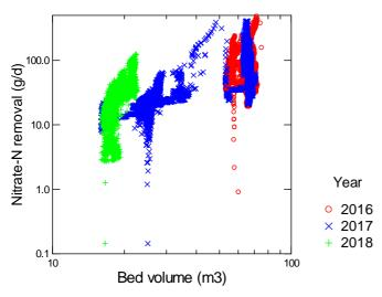
**Figure 9-1:** Relationship between nitrate-N removal rate and active bed volume by year. The active bed volume is the volume of bed submerged in water, as opposed to the total volume of woodchips.
