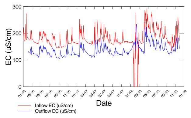
**Figure 6-2:** Comparison of hourly average inflow and outflow electrical conductivity. These values were derived from five-minute data.
