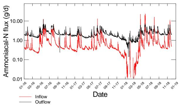
Figure 7-3: Comparison of woodchip filter inflow and outflow ammoniacal-N flux estimated using bootstrap regression models.
