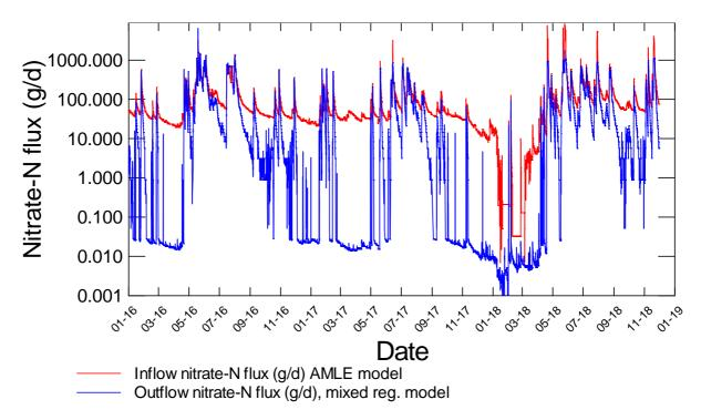
**Figure J-14:** Nitrate-N inflow and outflow flux from woodchip filter, estimated using two models. AMLE = model from LOADEST modelling package (Runkel et al. 2013), and the mixed regression model uses two relationships between discharge and concentration classified according to flow conditions. The relationship between model estimates and grab sample measurements are shown in Figure J-12.
