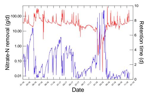
**Figure 7-10:** Relationship between nitrate-N removal (blue), estimated as the difference between inflow and outflow nitrate-N flux, and hydraulic retention time (grey). The inflow flux was estimated using the LOADEST AMLE model, and the outflow flux was estimated from inflow concentrations using the process described in section 2.5.2. These data are hourly average values.
