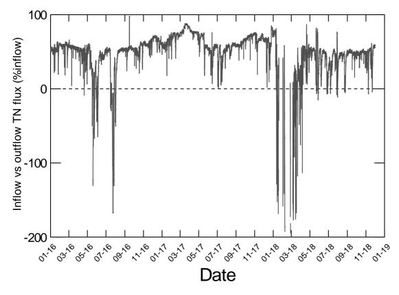
Figure J-18: Efficacy of TN removal by woodchip filter, expressed as proportion of inflow flux removed, estimated using bootstrap regression models.
