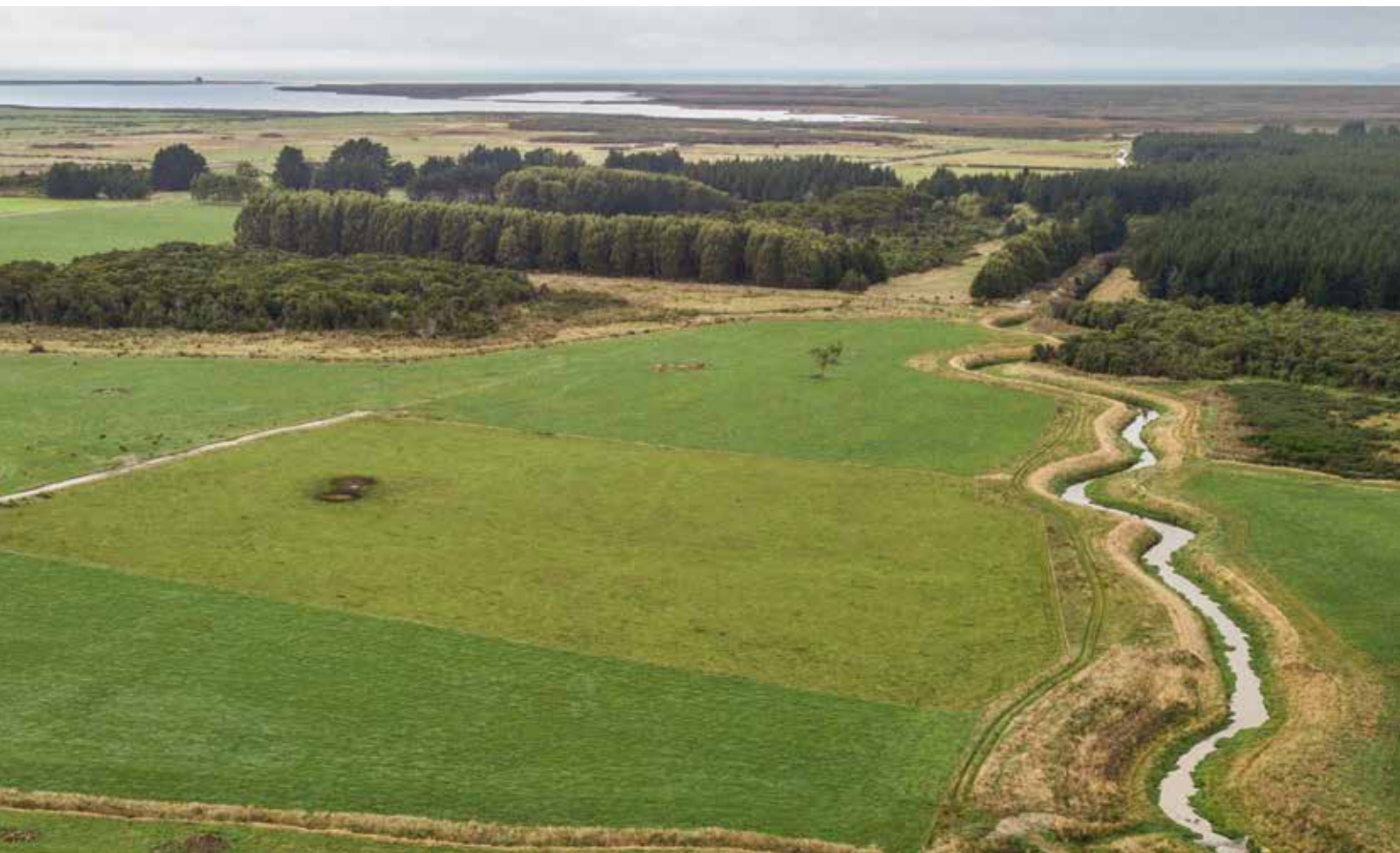
Waituna Creek looking south towards the Lagoon, showing areas where the two stage channels, instream habitat structures and plantings were undertaken, along with the Marshall Road property purchase
