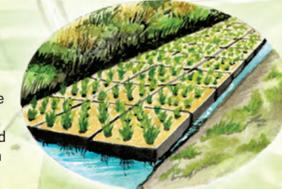
**Progress:** Monitoring has shown that nutrient uptake has been inconsistent - depending on the season and water levels. A key lesson learned for improving performance is greatly increasing the length of the wetland to 800m<sup>2</sup> to allow more time for the water to be filtered and the plant's roots and tops need to be trimmed regularly or plants replaced at least yearly to prevent dead growth from going back into the waterway.
