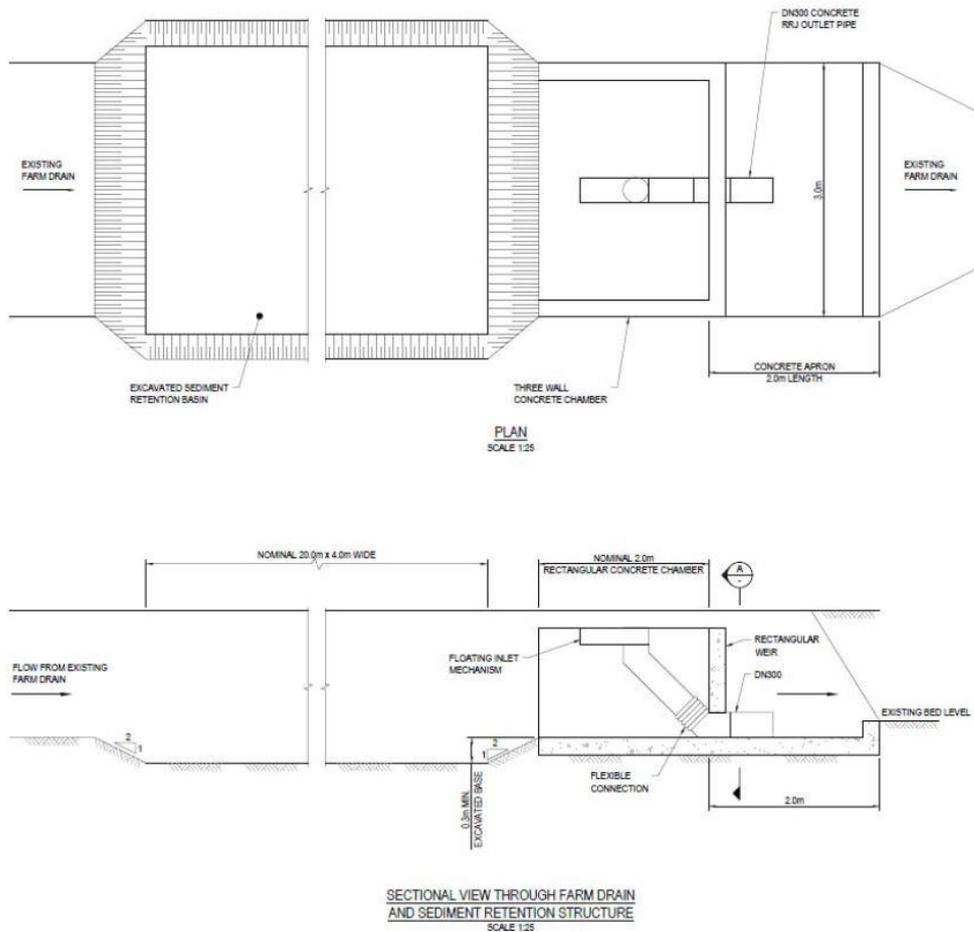
Figure 30: Schematic of Peak Run-off Control / Sediment Retention structure for farm drains
