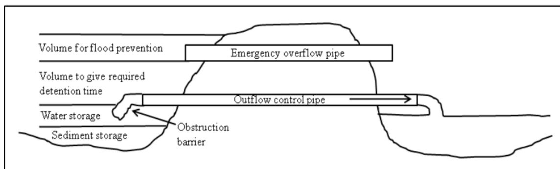
Figure 25: Generic schematic section of a peak runoff control structure
