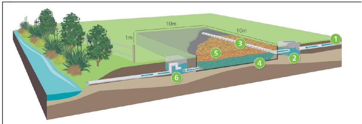
Figure 28: Schematic diagram of the woodchip bio-reactor near Oteramika
