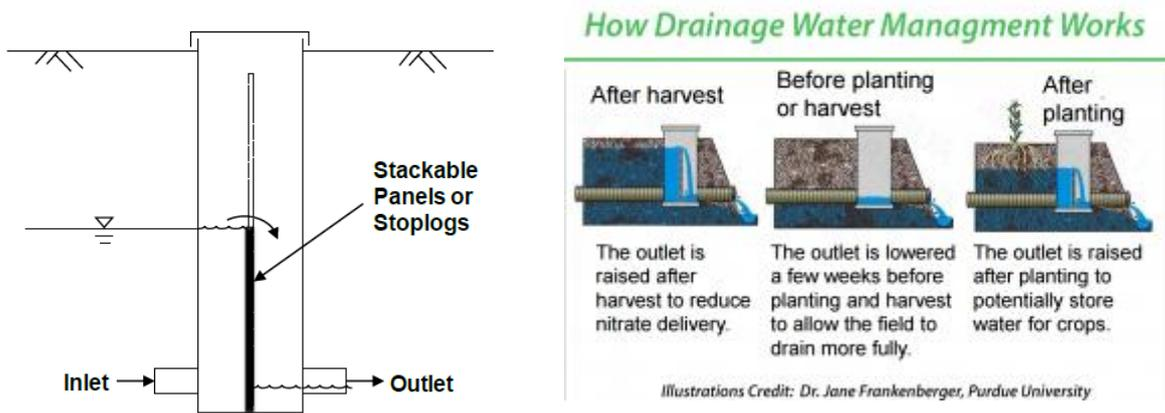
Figure 26: Schematic of how controlled drainage (or drainage water management) works
