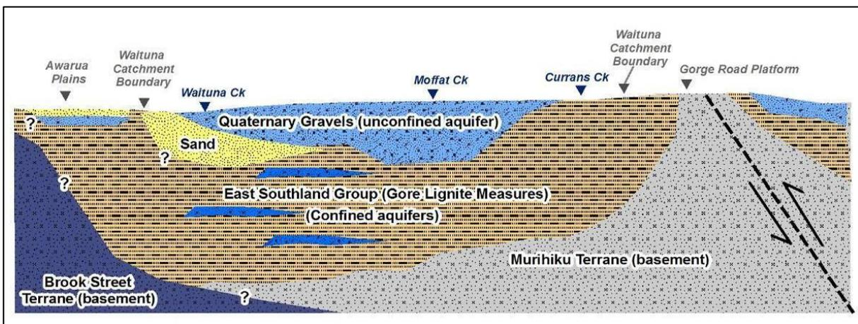
Figure 7: Schematic hydrogeological cross-section of the Waituna catchment
