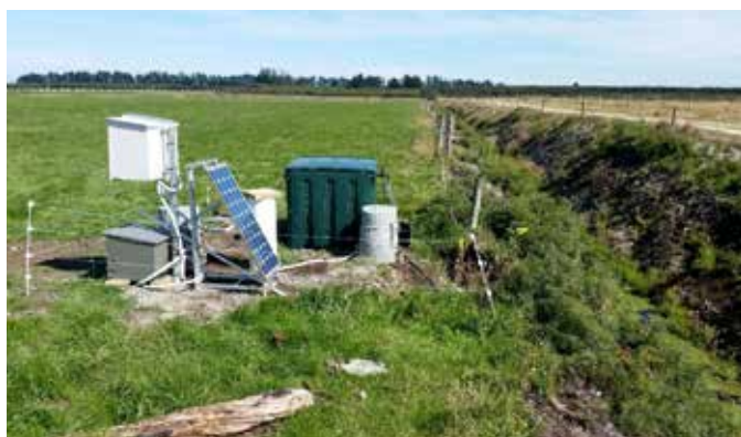
Phosphorous passive filter installed on private land. Aluminised zeolite will help remove phosphates from tile drains prior to entering into waterways.
